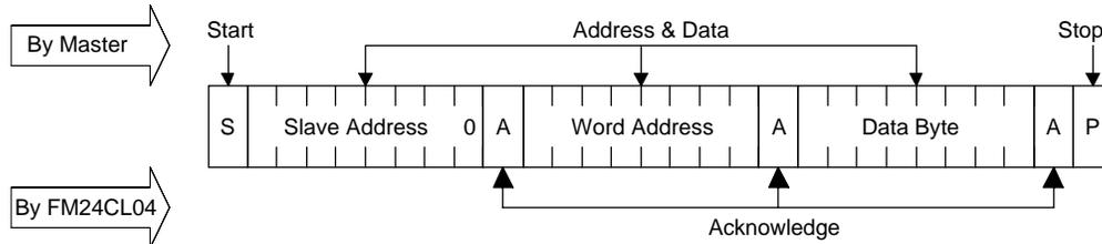
Figure 5. Byte Write
