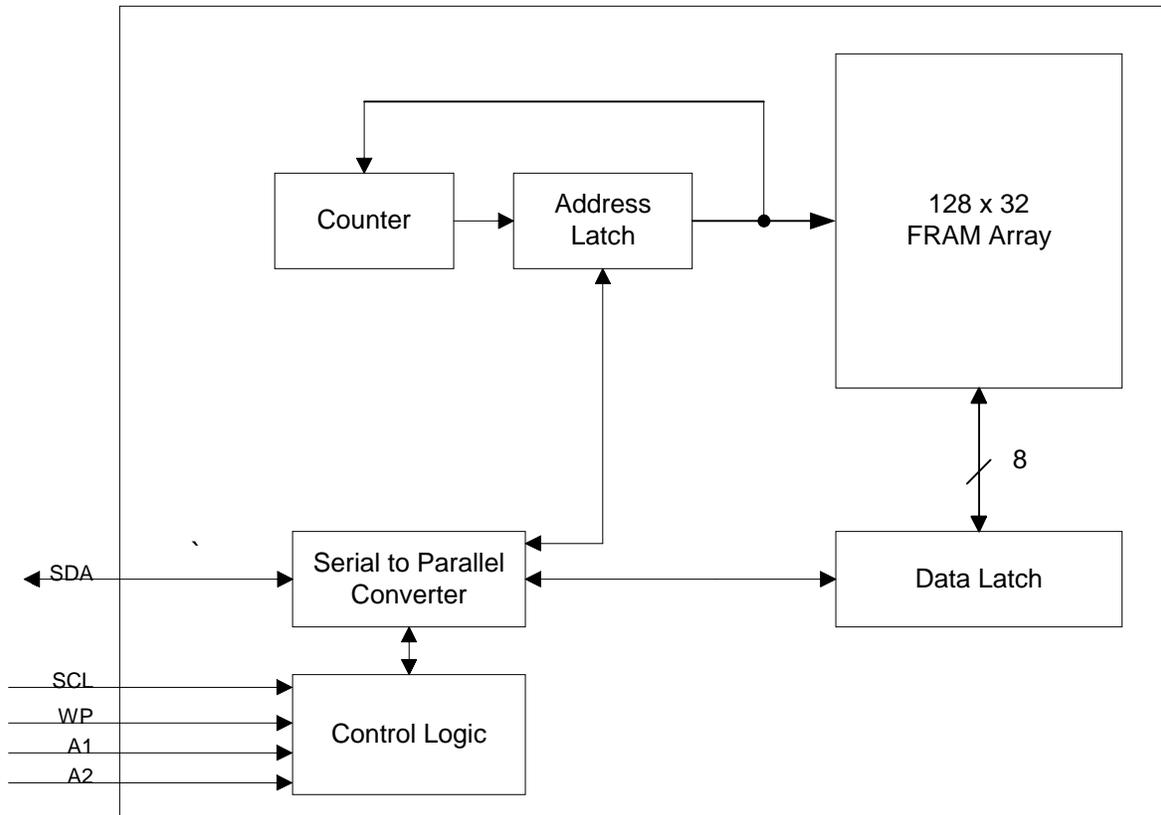
Figure 1. Block Diagram
