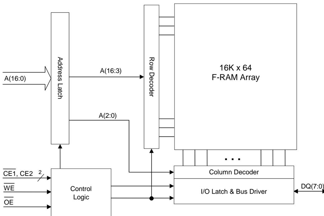
Figure 1. Block Diagram
