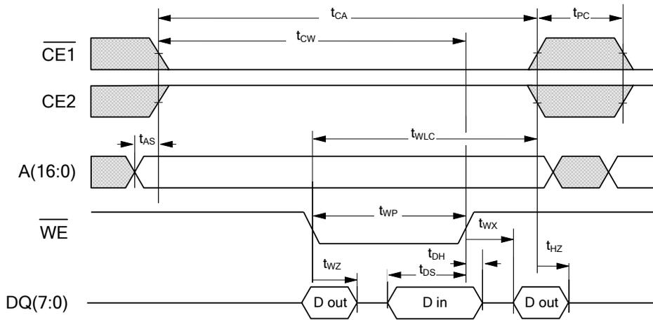
Write Cycle Timing 2 (/CE-Controlled)
