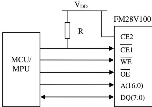
Figure 3. Typical Application using Pullup Resistor on  $\overline{CE1}$
