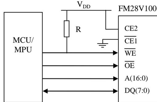
Figure 4. Use of Pullup Resistor on  $\overline{WE}$
