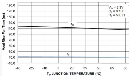
Figure 18.  $V_{OUT}$  Rise/Fall Time vs. Temperature ( $R_L=500\ \Omega$ )
