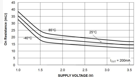
**Figure 15. R<sub>ON</sub> vs. Supply Voltage**
