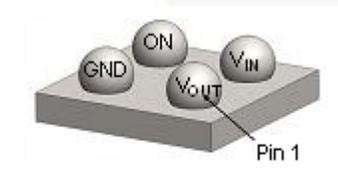
Figure 4. 1 x 1 mm WLCSP Bumps Facing Up
