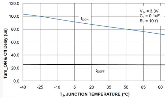
Figure 17.  $V_{OUT}$  Turn-On/Turn-Off Delays vs. Temperature ( $R_L=10\ \Omega$ )
