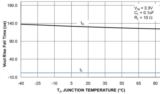
Figure 16.  $V_{OUT}$  Rise/Fall Times vs. Temperature ( $R_L=10\ \Omega$ )
