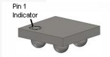
Figure 3. 1 x 1 mm WLCSP Bumps Facing Down
