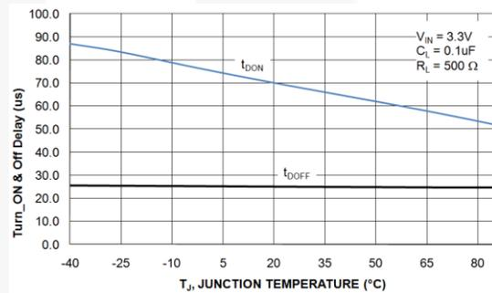
Figure 19.  $V_{OUT}$  Turn-On/Turn-Off Delays vs. Temperature ( $R_L=500\ \Omega$ )
