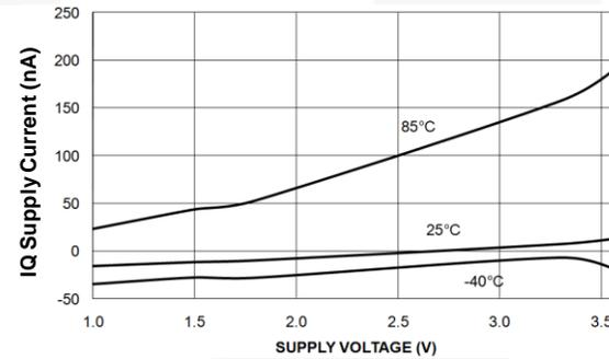
**Figure 13. Quiescent Current vs. Supply Voltage (V<sub>ON</sub>=V<sub>IN</sub>)**
