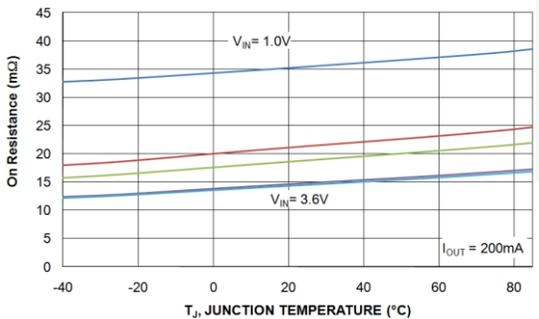
**Figure 14. R<sub>ON</sub> vs. Temperature**
