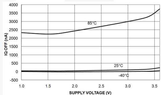
**Figure 11. Off Supply Current vs. Supply Voltage**
