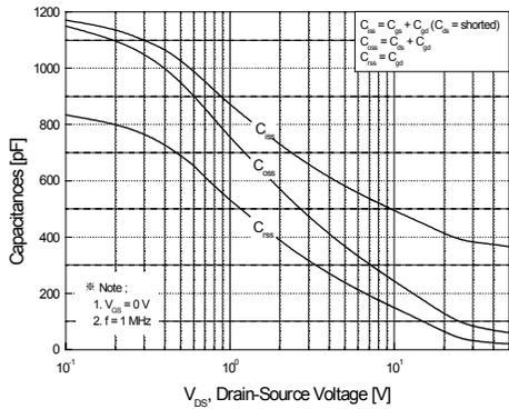
Figure 5. Capacitance Characteristics
