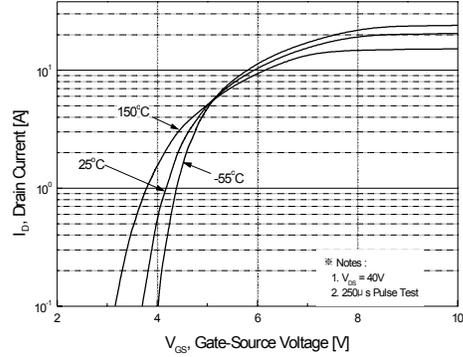
Figure 2. Transfer Characteristics
