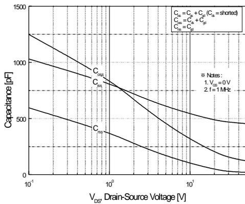
Figure 5. Capacitance Characteristics
