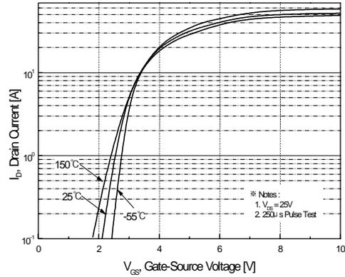
Figure 2. Transfer Characteristics
