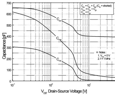
**Figure 5. Capacitance Characteristics**
