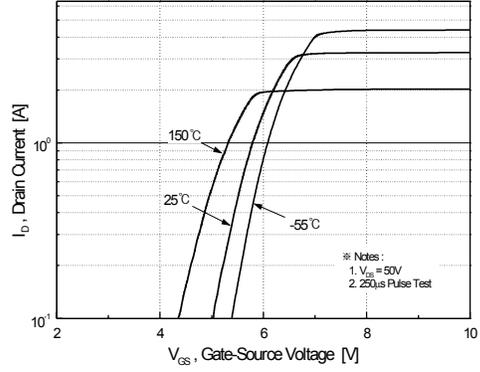
**Figure 2. Transfer Characteristics**
