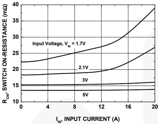
Figure 6. Switch On Resistance vs. Switch Current
