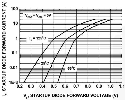
**Figure 12. Startup Diode Current vs. Forward Voltage**
