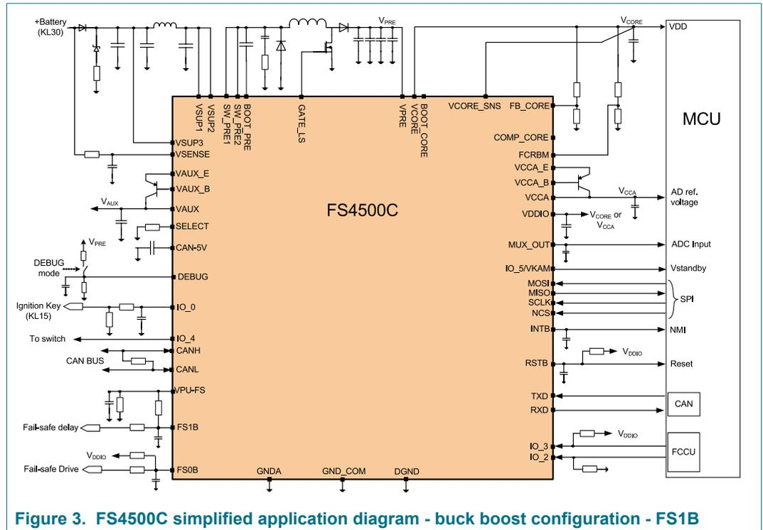
Figure 3. FS4500C simplified application diagram - buck boost configuration - FS1B
