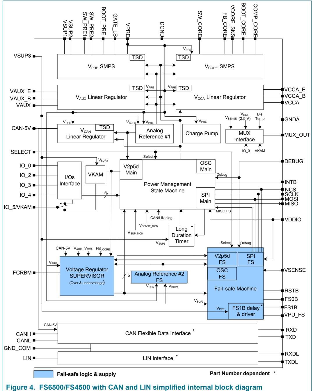
Figure 4. FS6500/FS4500 with CAN and LIN simplified internal block diagram
