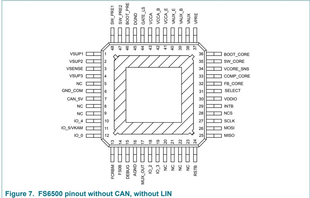
Figure 7. FS6500 pinout without CAN, without LIN
