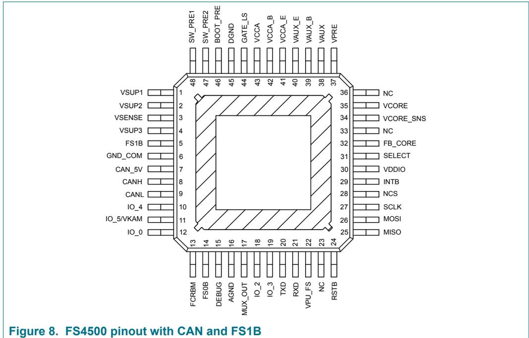
Figure 8. FS4500 pinout with CAN and FS1B
