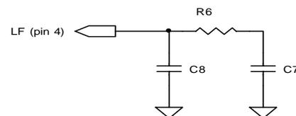
**Table 2. FS781/82/84 Recommended Loop Filter Values C7 (pF) @ +3.3 VDC ±5% (R6 = 3.3K)<sup>[1, 2, 3, 4]</sup>**
