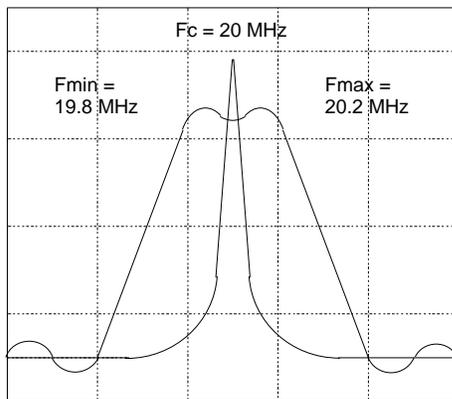
**Figure 3. Spectrum Analysis of 19.8 – 20.2 MHz Clock**
