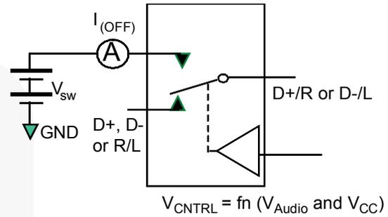
**Figure 12. Off Leakage**
