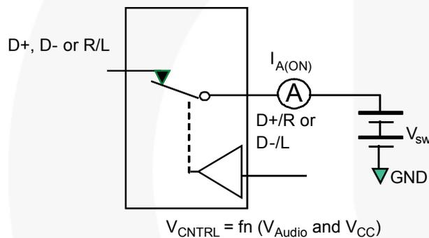
**Figure 13. On Leakage**
