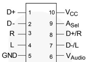
Figure 3. 10-Pin MSOP
