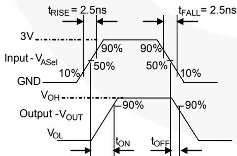
**Figure 15. Turn-On / Turn-Off Waveforms ( $A_{Sel}$ )**
