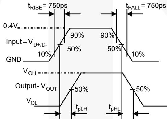
Figure 18. Pulse Skew:  $t_{SK(P)} = | t_{pHL} - t_{pLH} |$
