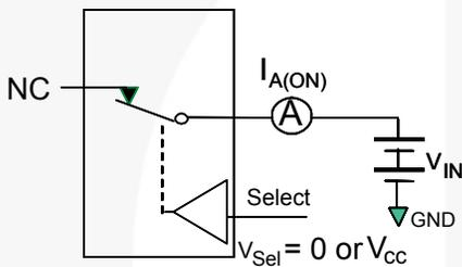
Figure 5. On Leakage
