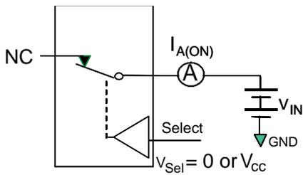
Figure 5. On Leakage
