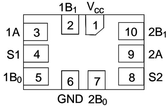
Figure 2. 10-Pin UMLP (Top Through View)
