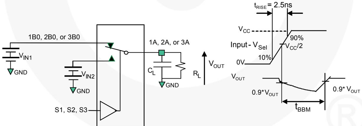
$R_L$  and  $C_L$  are functions of the application environment (see AC Tables for specific values)
