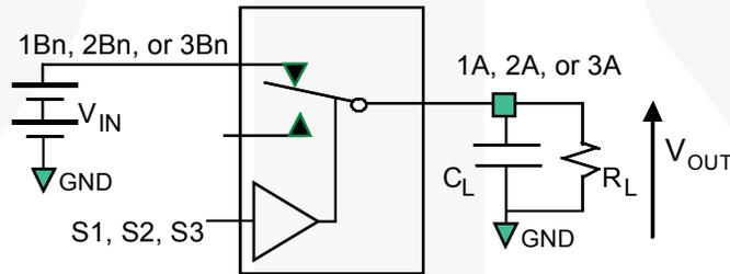
$R_L$  and  $C_L$  are functions of the application environment (see AC Tables for specific values)
