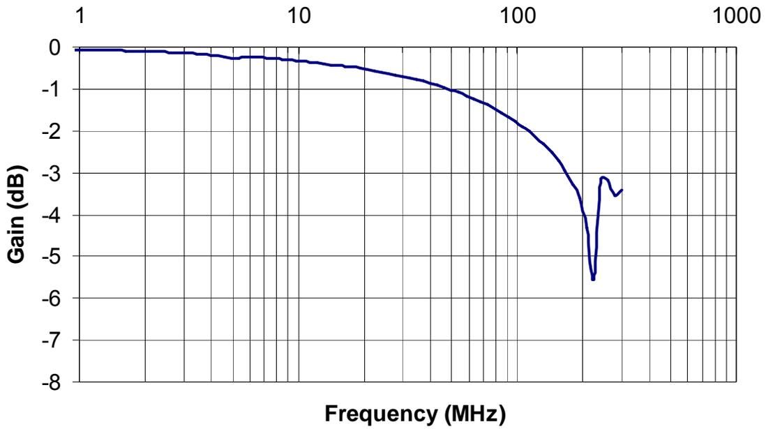
**Figure 6.** Bandwidth Characterization, Frequency Response at  $V_{CC}=3.3V$ ,  $C_L=0pF$
