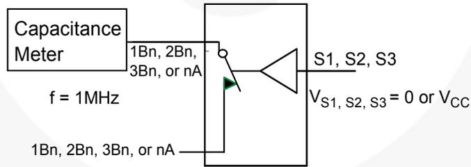
**Figure 19. Channel On Capacitance**
