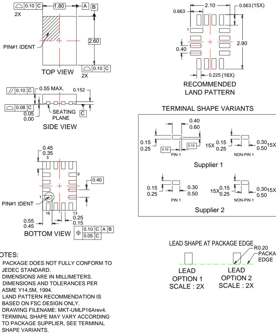
Figure 10. 16-Pin Ultrathin Molded Leadless Package (UMLP)
