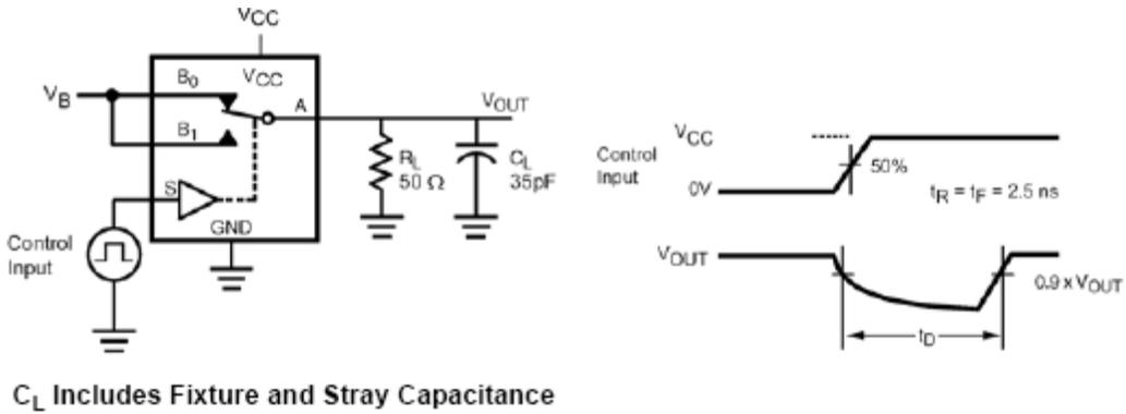
Figure 4. Break-Before-Make Timing
