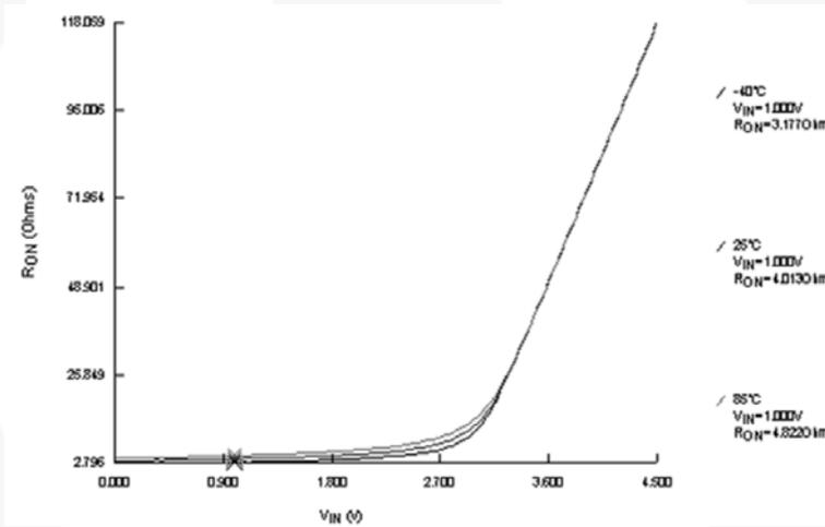
Figure 9. R<sub>ON</sub> Switch On Resistance, I<sub>ON</sub>=13mA
