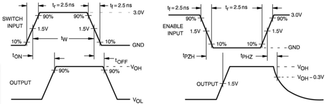
Figure 12. AC Waveforms
