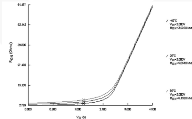
Figure 10. R<sub>ON</sub> Switch On Resistance, I<sub>ON</sub>=26mA
