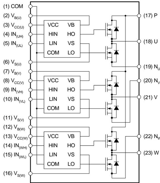
**Note:** Source terminal of each MOSFET is not connected to supply ground or bias voltage ground inside SPM. External connections should be made as indicated in Figure 2 and 5.
