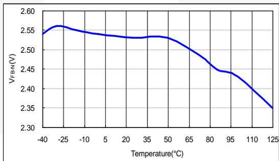
Figure 19. V<sub>FB-N</sub> vs. Temperature
