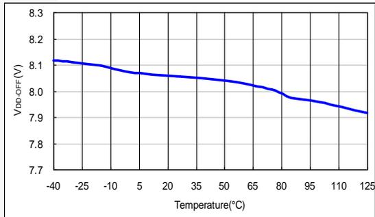
**Figure 9. V<sub>DD-OFF</sub> vs. Temperature**
