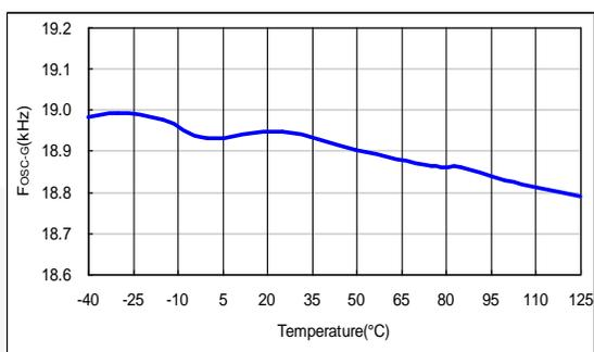
Figure 15. f<sub>osc-g</sub> vs. Temperature
