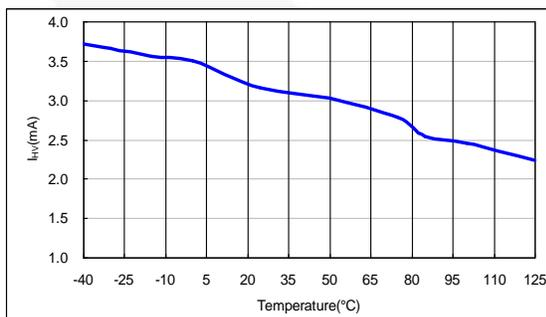
**Figure 12. I<sub>HV</sub> vs. Temperature**
