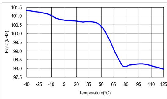
Figure 14. f<sub>osc</sub> vs. Temperature
