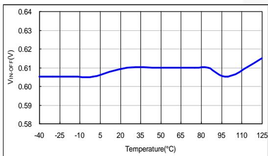
Figure 16. V<sub>IN-OFF</sub> vs. Temperature
