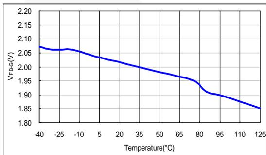
Figure 20. V<sub>FB-G</sub> vs. Temperature
