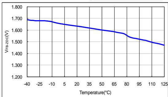
Figure 21. V<sub>FB-ZDC</sub> vs. Temperature
