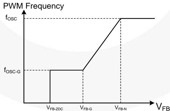
**Figure 5. V<sub>FB</sub> vs. PWM Frequency**
