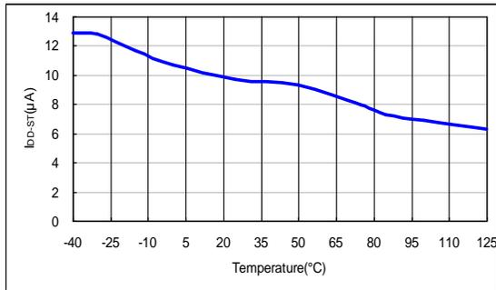
**Figure 6. I<sub>DD-ST</sub> vs. Temperature**
