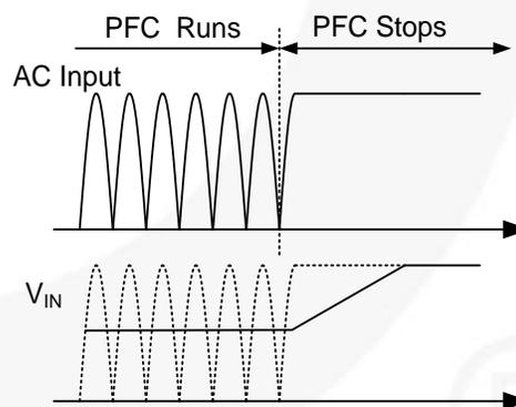
Figure 25.  $V_{IN}$  Level According to PFC Operation
