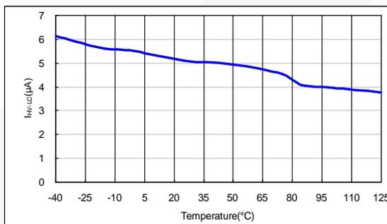
**Figure 13. I<sub>HV-LC</sub> vs. Temperature**
