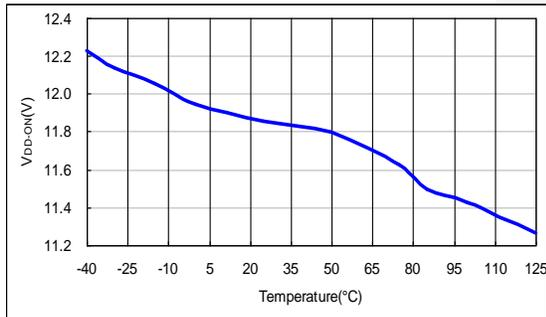
**Figure 8. V<sub>DD-ON</sub> vs. Temperature**
