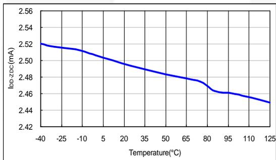
Figure 18. I<sub>DD-ZDC</sub> vs. Temperature
