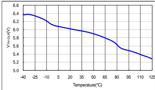
**Figure 10. V<sub>TH-OLP</sub> vs. Temperature**
