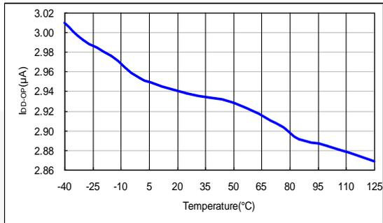
**Figure 7. I<sub>DD-OP</sub> vs. Temperature**
