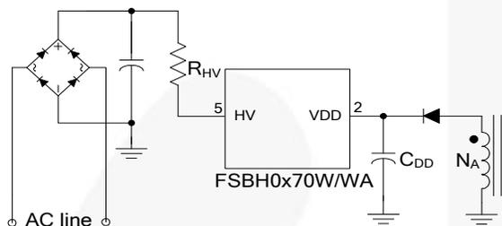
Figure 22. Startup Circuit
