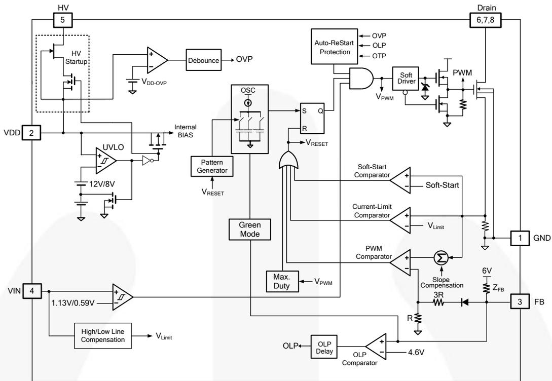
Figure 2. FSBH0170W / 0270W Internal Block Diagram
