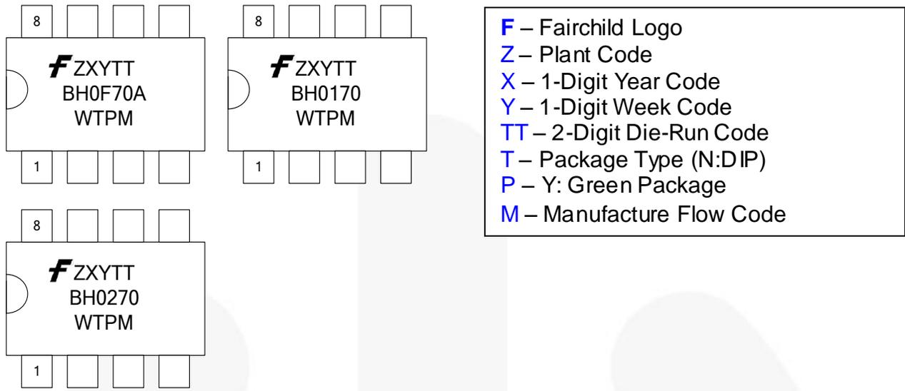
Figure 4. Pin Configuration and Top Mark Information
