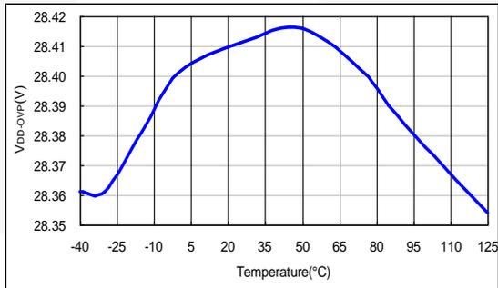
**Figure 11. V<sub>DD-OVP</sub> vs. Temperature**
