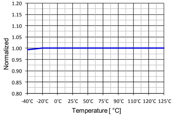
Figure 12. UVLO Threshold Voltage ( $V_{STOP}$ ) vs.  $T_A$
