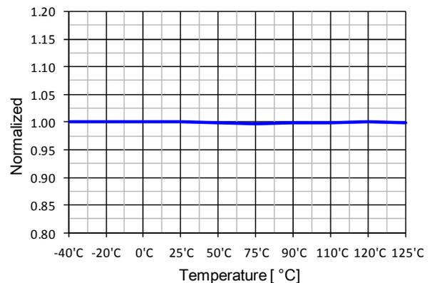
Figure 16. Maximum Duty Ratio ( $D_{MAX}$ ) vs.  $T_A$
