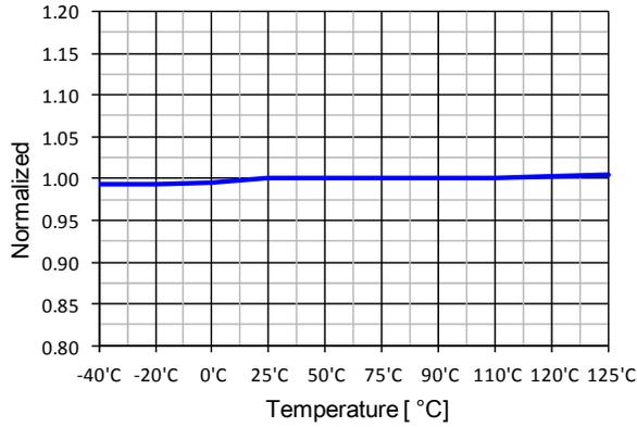
Figure 11. UVLO Threshold Voltage ( $V_{START}$ ) vs.  $T_A$
