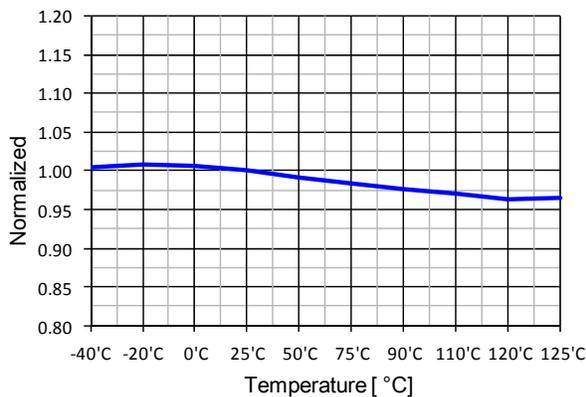
Figure 15. Switching Frequency ( $f_s$ ) vs.  $T_A$
