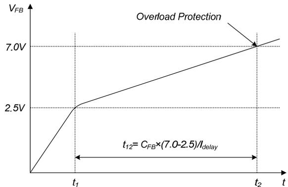
**Figure 20. Overload Protection**
