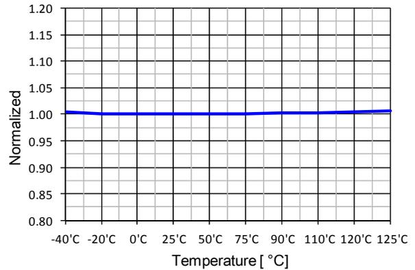
Figure 14. Over-Voltage Protection ( $V_{OVP}$ ) vs.  $T_A$
