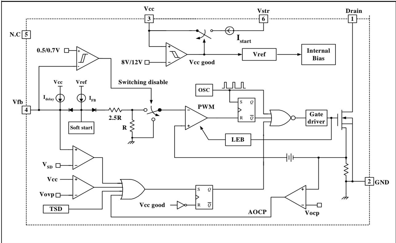
Figure 2. Functional Block Diagram of FSDM07652R
