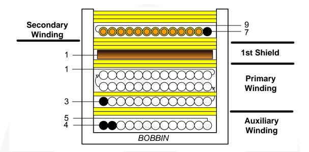
Figure 33. Transformer Specification
