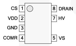
Figure 5. Pin Configuration
