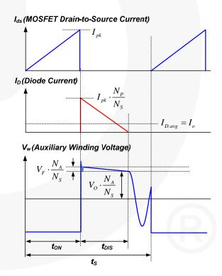
Figure 25. Key Waveforms of DCM Flyback
