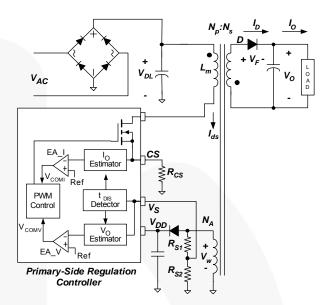
Figure 24. Simplified PSR Flyback Converter Circuit
