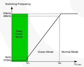
Figure 26. Switching Frequency in Green Mode
