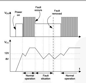
Figure 17. Auto-Restart Protection Waveforms
