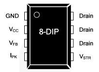
Figure 3. Pin Configuration
