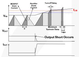
Figure 20. Output Short Waveforms (OSP)
