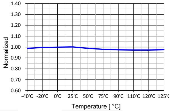
Figure 6. Operating Switching Current ( $I_{OPS}$ ) vs.  $T_A$
