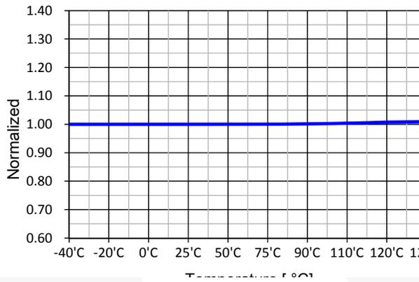
Figure 13. Shutdown Feedback Voltage ( $V_{SD}$ ) vs.  $T_A$
