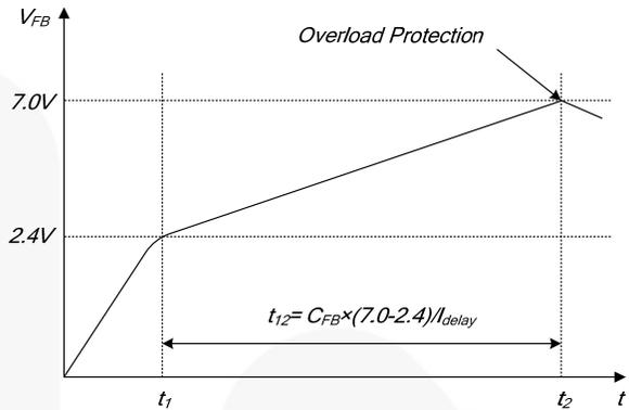
**Figure 20. Overload Protection**
