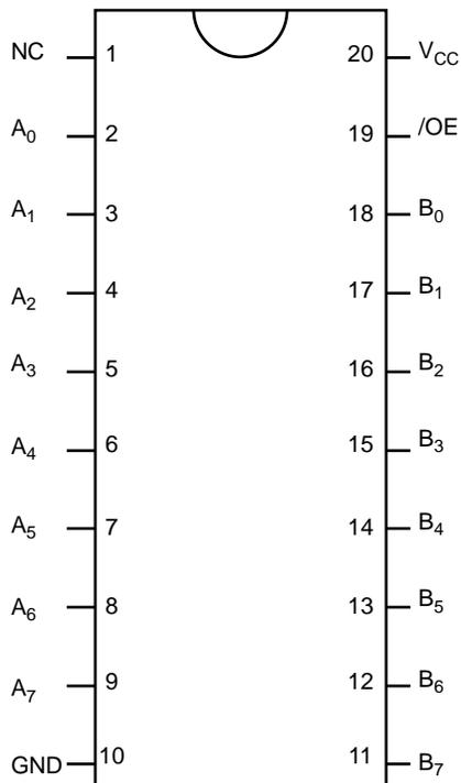
Figure 2. Pin Configuration
