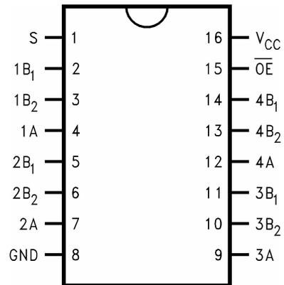
Figure 2. Connection Diagram
