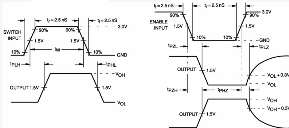
**Figure 4. AC Waveforms**
