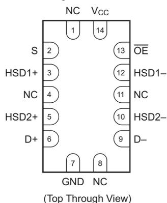
Pin Assignment for MSOP
