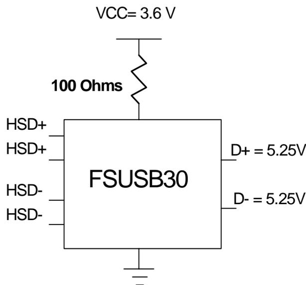
**Figure 17. Adding 100Ω resistor in series with the V<sub>CC</sub> supply allows the FSUSB30 to withstand a Vbus short when powered up**
