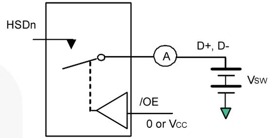
**Figure 6. Off/On Leakage**
