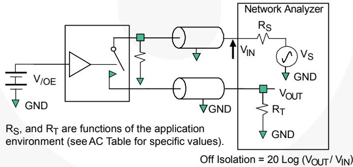
$R_S$ , and  $R_T$  are functions of the application environment (see AC Table for specific values).
