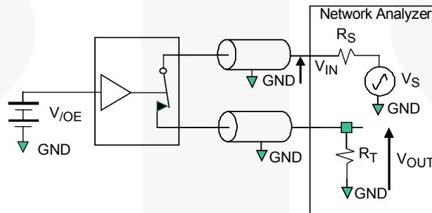
$R_S$ , and  $R_T$  are functions of the application environment (see AC Table for specific values).
