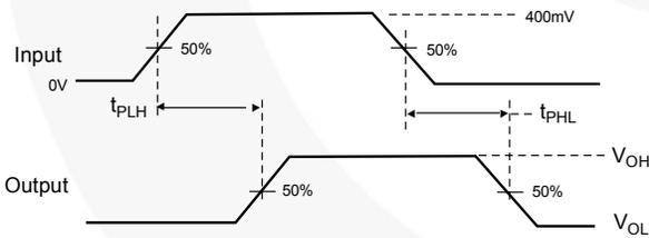
**Figure 9. Propagation Delay ( $t_{rF} - 500ps$ )**
