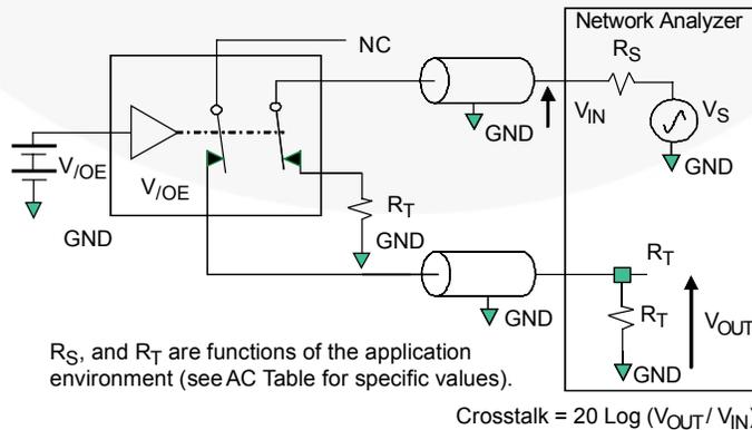
$R_S$ , and  $R_T$  are functions of the application environment (see AC Table for specific values).
