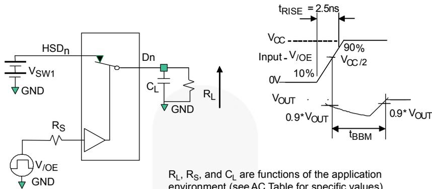
$R_L$ ,  $R_S$ , and  $C_L$  are functions of the application environment (see AC Table for specific values).  $C_L$  includes text figure and stray capacitance.
