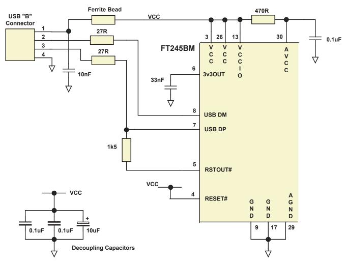
Figure 7 illustrates a typical USB bus powered configuration. A USB Bus Powered device gets its power from the USB bus. Basic rules for USB Bus power devices are as follows –
