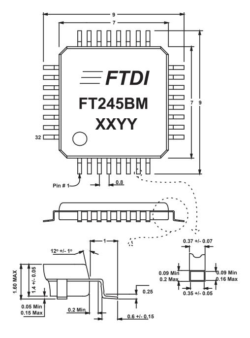
The FT245BM is supplied in a 32 LD LQFP package as standard. This package has a 7mm x 7mm body (9mm x 9mm including leads) with leads on a 0.8mm pitch. An alternative 5mm x 5mm leadless chip scale package is available on special request for projects where package area is critical.
