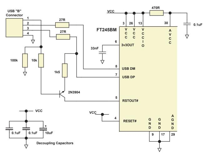
Figure 8 illustrates a typical USB self powered configuration. A USB Self Powered device gets its power from its own POWER SUPPLY and does not draw current from the USB bus. Basic rules for USB Self power devices are as follows
