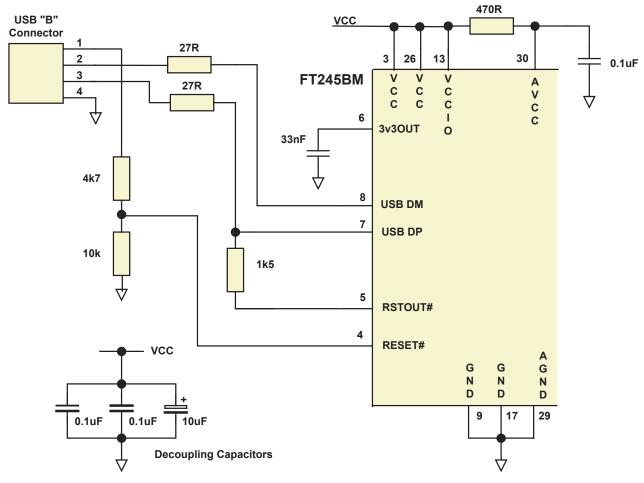
Figure 9 illustrates a variant of the circuit shown in Figure 8. This time, the 1k5 pull-up resistor on USB DP is connected to RSTOUT# as per the bus-power circuit. However, the USB Bus Power is used to control the RESET# Pin of the FT245BM device. When the USB Host or Hub power is off, RESET# will go low and the device will be held in reset. As RESET# is low, RSTOUT# will also be low, so no current will be forced down USB DP via the 1k5 pull-up resistor.
