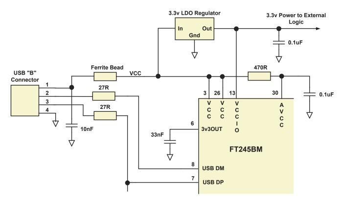
Figure 10 shows how to configure the FT245BM to interface with a 3.3v logic device. In this example, a discrete 3.3v regulator is used to supply the 3.3v logic from the USB supply. VCCIO is connected to the output of the 3.3v regulator, which in turn will cause the FIFO interface IO pins to drive out at 3.3v level. For USB bus powered circuits some considerations have to be taken into account when selecting the regulator –
