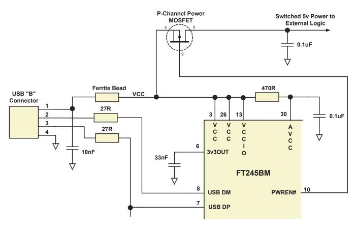
USB Bus powered circuits need to be able to power down in USB suspend mode in order to meet the <= 500uA total suspend current requirement (including external logic). Some external logic can power itself down into a low current state by monitoring the POWEREN# pin. For external logic that cannot power itself down in that way, the FT245BM provides a simple but effective way of turning off power to external circuitry during USB suspend.
