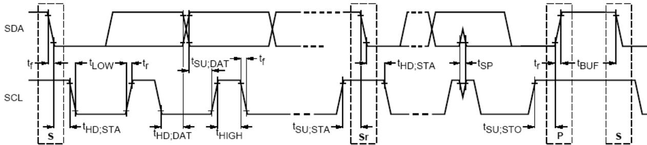
Figure 4. Definition of Timing for Full-Speed Mode Devices on the I<sup>2</sup>C Bus
