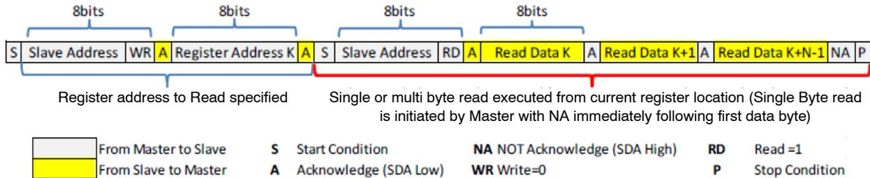
NOTE: If Register is not specified Master will begin read from current register. In this case only sequence showing in Red bracket is needed.
