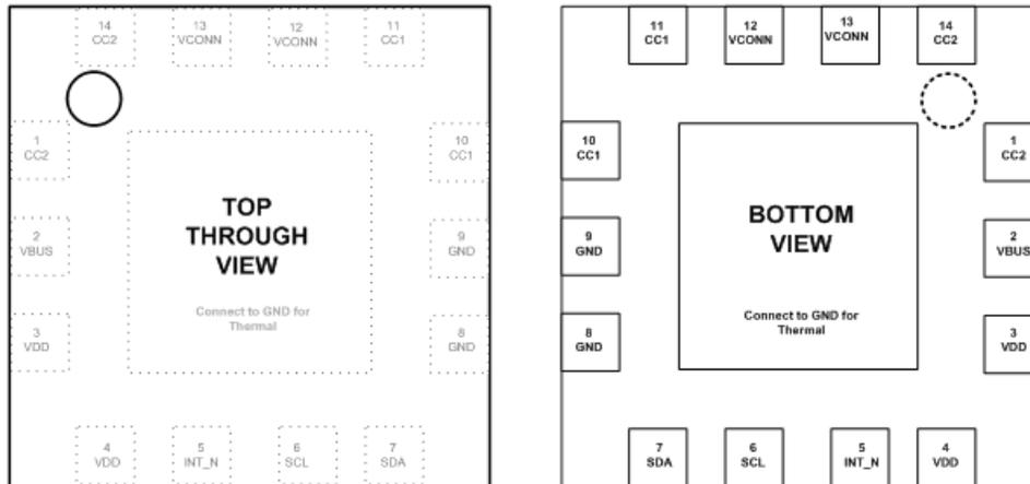
Figure 4. FUSB302TMPX Pin Assignment (N/C = No Connect)
