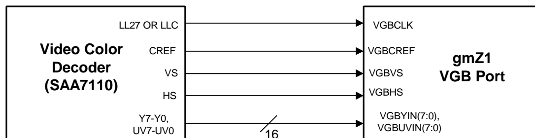
Figure 4: Video Color Decoder Connection to gmZ1
