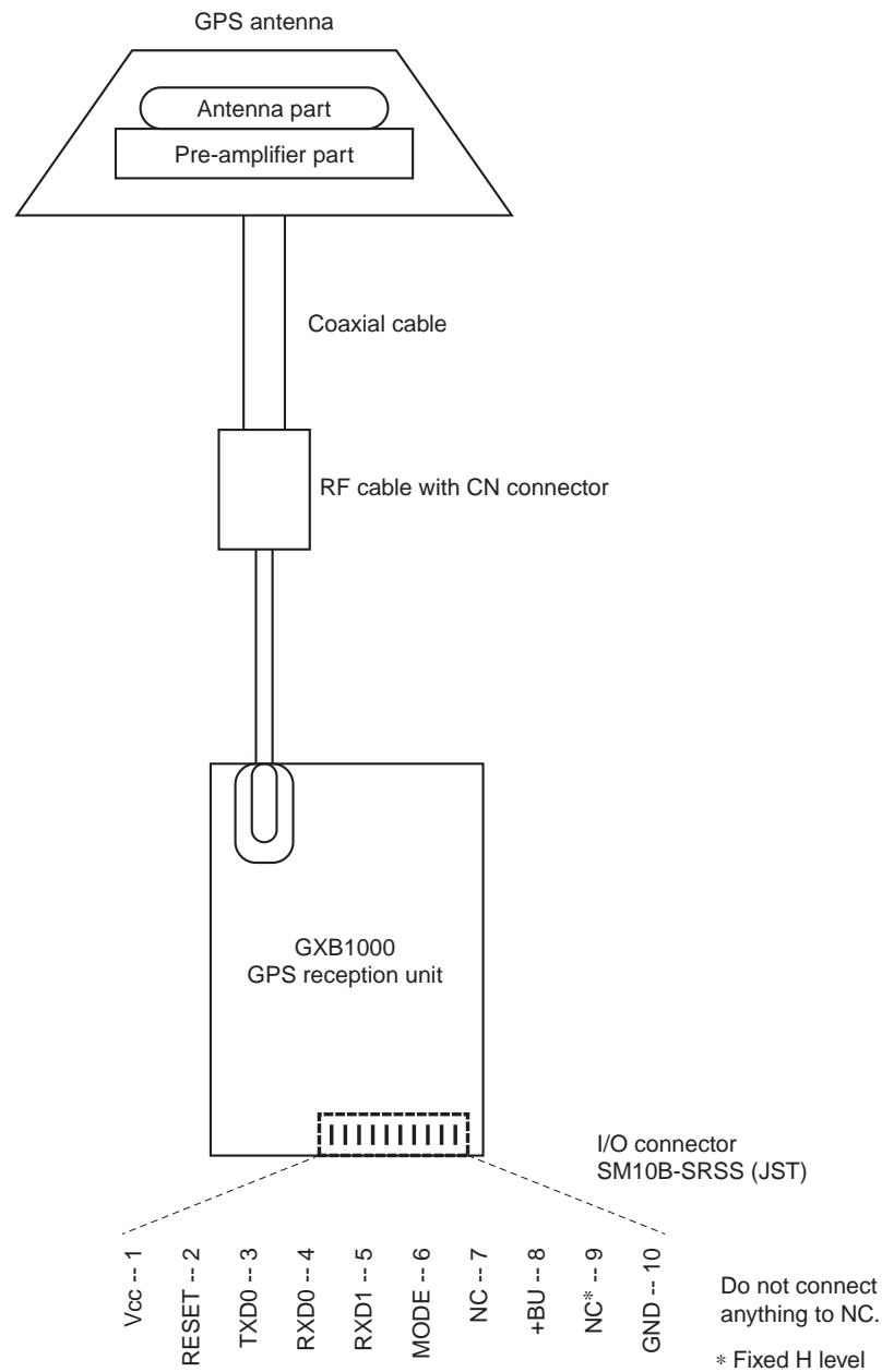
**GXB1000 GPS Reception Unit External Figure (Connector type)****Specification of form name**
