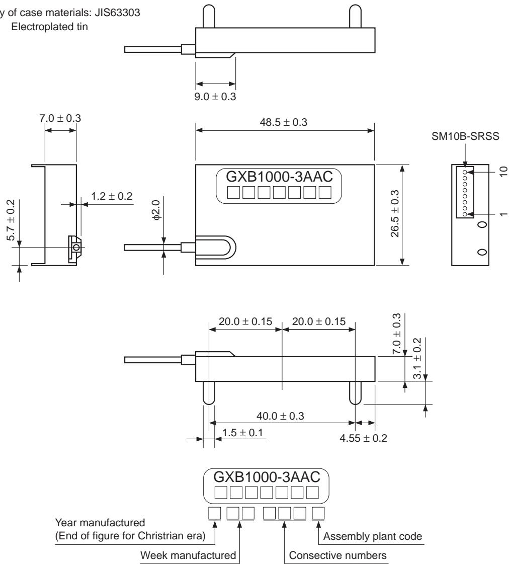
GXB1000 GPS Reception Unit External Figure (Pin type)
