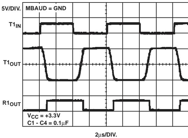
FIGURE 6. LOOPBACK TEST AT 250kbps ( $C_L = 1000\text{pF}$ )
