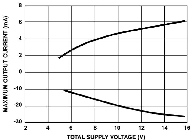
FIGURE 9. MAXIMUM OUTPUT CURRENT vs SUPPLY VOLTAGE
