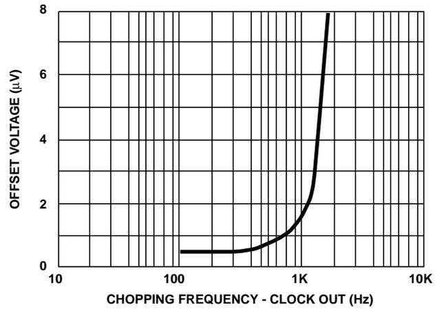
FIGURE 14. INPUT OFFSET VOLTAGE vs CHOPPING FREQUENCY
