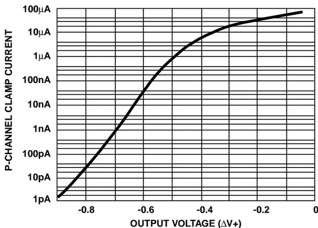
FIGURE 21. P-CHANNEL CLAMP CURRENT vs OUTPUT VOLTAGE
