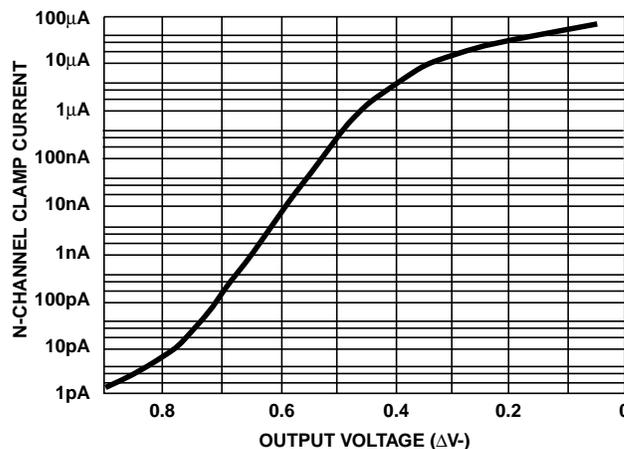
FIGURE 20. N-CHANNEL CLAMP CURRENT vs OUTPUT VOLTAGE
