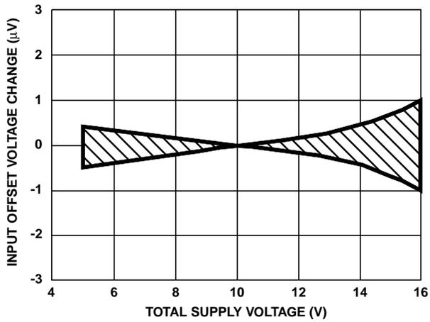
FIGURE 13. INPUT OFFSET VOLTAGE CHANGE vs SUPPLY VOLTAGE
