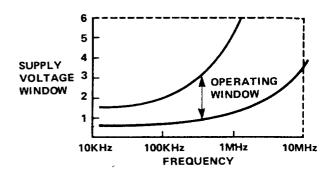
For example, if instead of 6.5MHz, a 1MHz oscillator is required, it is recommended that the supply voltage be reduced to between 2 and 2.5 volts. This may be realized by using a series resistor in series with the 5V positive supply line plus a decoupling capacitor. The quartz crystal parameters, etc., will determine the value of this resistor NOTE Except for the output open drain n-channel transistors no other terminal is permitted to exceed the supply voltage limits.
