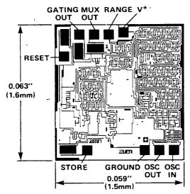
Chip may be die attached using conventional eutectic or epoxy procedures. Wire bonding may be either aluminum ultrasonic or gold compression.
