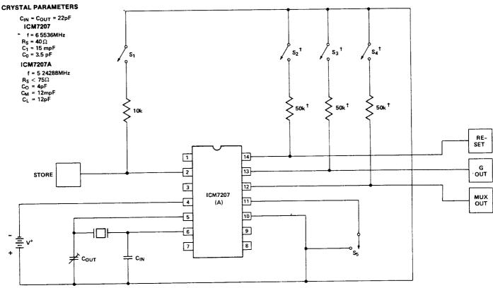
SWITCHES  $s_1,\,s_2,\,s_3,\,s_4$  open circuit for supply current measurement switch  $\,s_5$  open circuit for slow gating period
