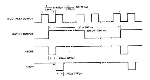
Referring to the test circuit, the crystal oscillator frequency is divided by  $2^{12}$  to provide both the multiplex frequency and generate the output pulse widths. The GATING OUTPUT
