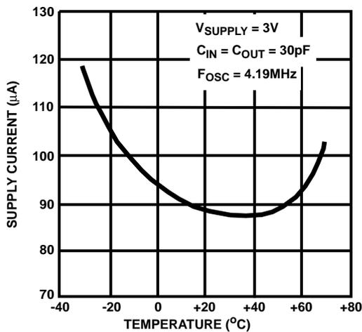
FIGURE 3. SUPPLY CURRENT AS A FUNCTION OF TEMPERATURE
