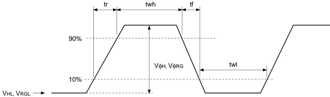
(4) Substrate clock waveform
