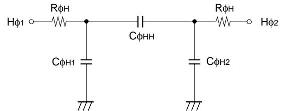
**Horizontal transfer clock equivalent circuit**
