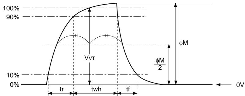
(2) Vertical transfer clock waveform
