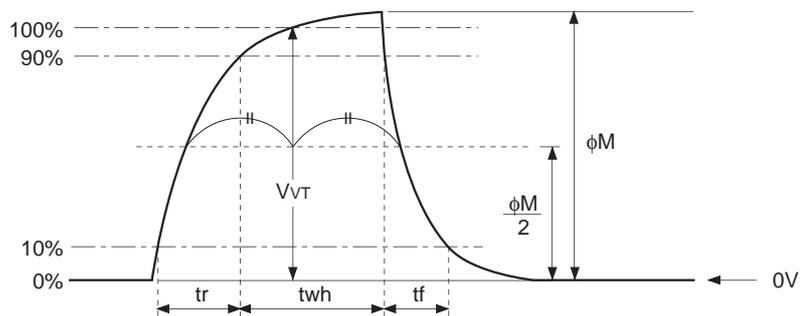
(2) Vertical transfer clock waveform
