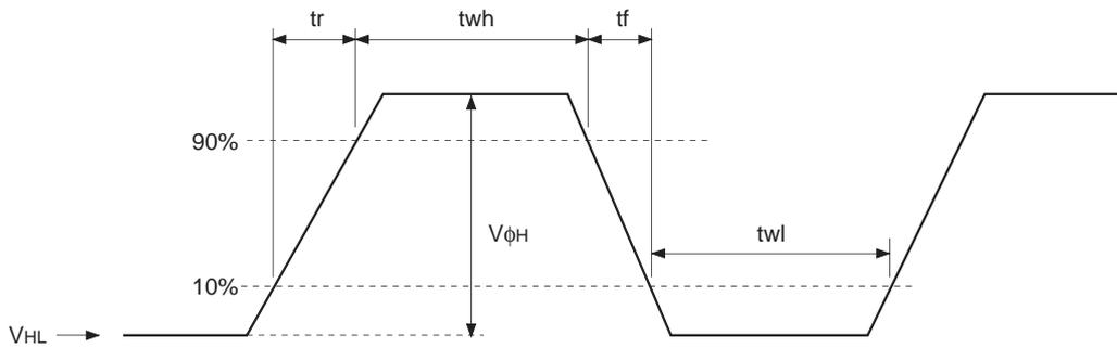
**(4) Reset gate clock waveform**
