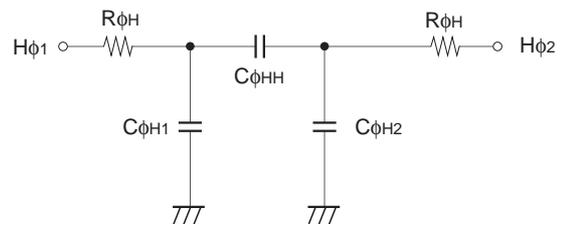
**Horizontal transfer clock equivalent circuit**
