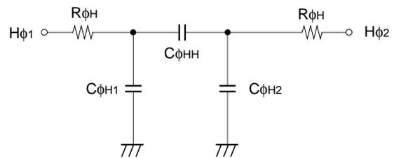
**Horizontal transfer clock equivalent circuit**
