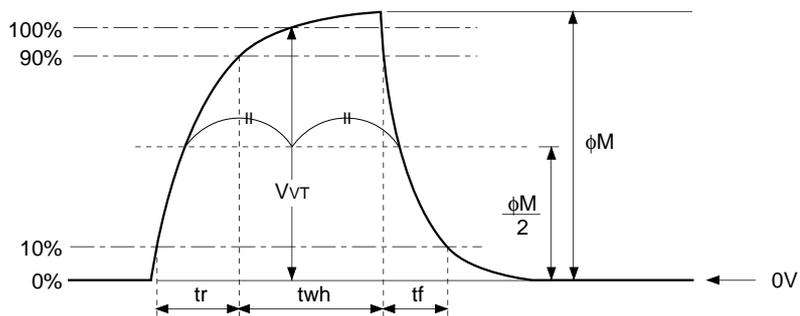
(2) Vertical transfer clock waveform
