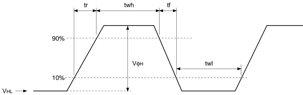
**(4) Reset gate clock waveform**
