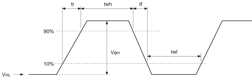
**(4) Reset gate clock waveform**
