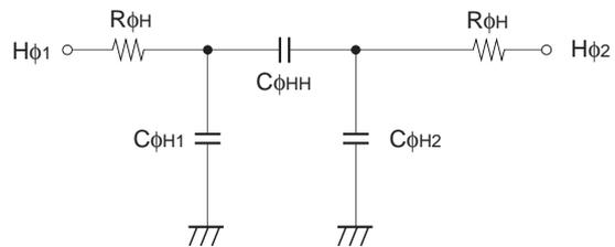
**Horizontal transfer clock equivalent circuit**
