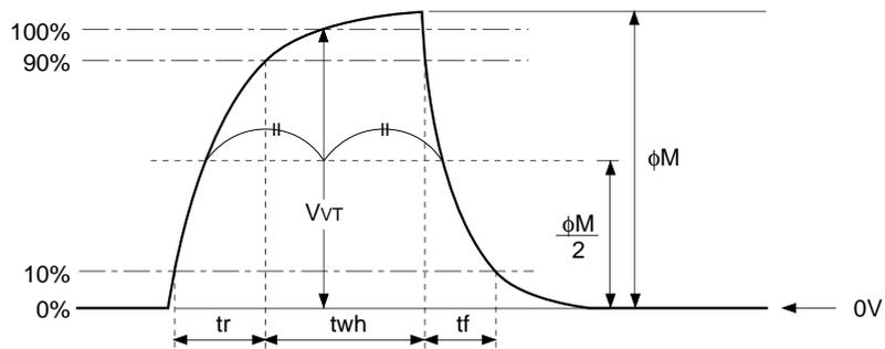
(2) Vertical transfer clock waveform
