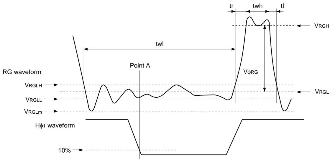
$V_{RGLH}$  is the maximum value and  $V_{RGLL}$  is the minimum value of the coupling waveform during the period from Point A in the above diagram until the rising edge of RG. In addition,  $V_{RGL}$  is the average value of  $V_{RGLH}$  and  $V_{RGLL}$ .
