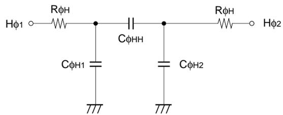
**Horizontal transfer clock equivalent circuit**
