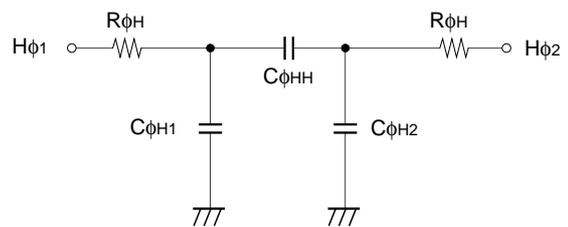
**Horizontal transfer clock equivalent circuit**
