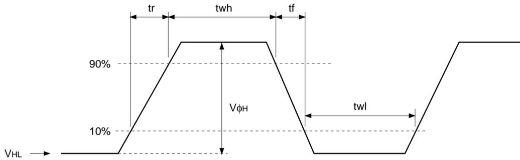
**(4) Reset gate clock waveform**
