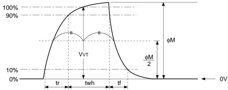
(2) Vertical transfer clock waveform
