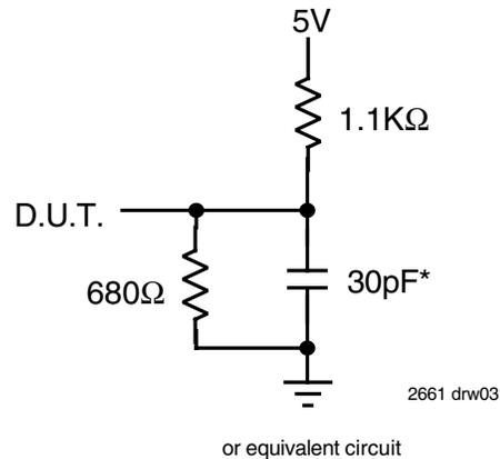
Figure 1. Output Load
