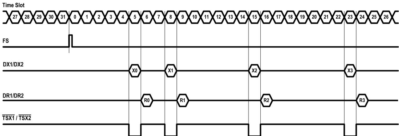
Figure - 10 Typical Frame Sync Timing (2 MHz Operation)
