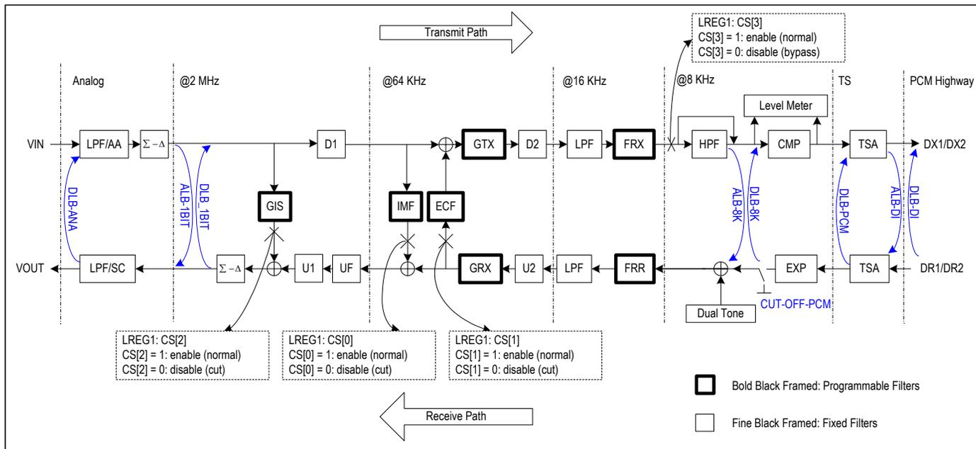
Figure - 4 Signal Flow for Each Channel
