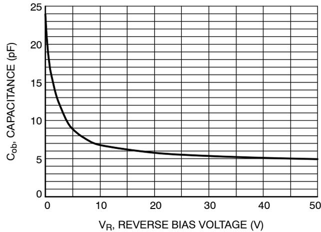
Figure 10. Output Capacitance
