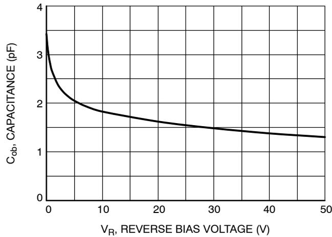
**Figure 5. Output Capacitance**
