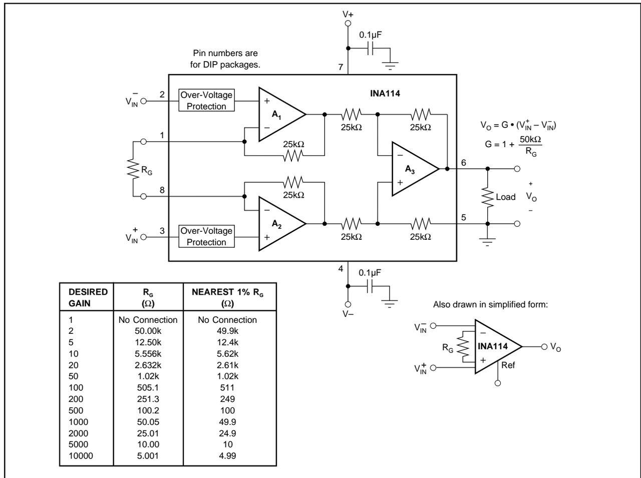
FIGURE 1. Basic Connections.
