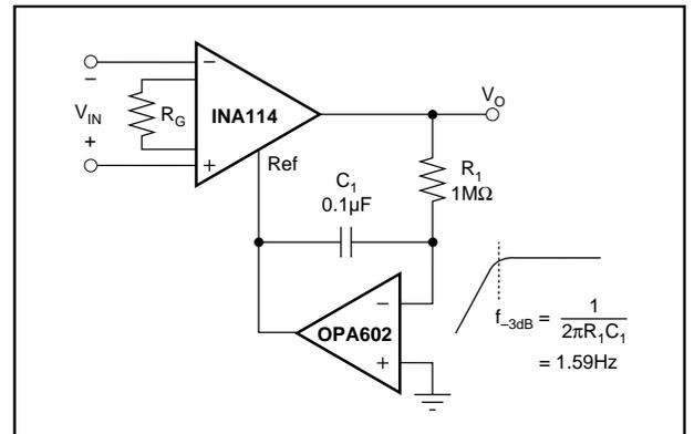
FIGURE 12. AC-Coupled Instrumentation Amplifier.
