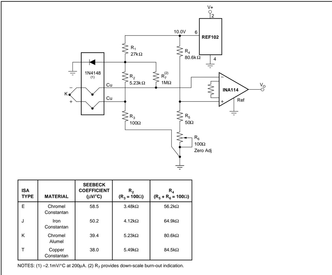
FIGURE 9. Thermocouple Amplifier With Cold Junction Compensation.
