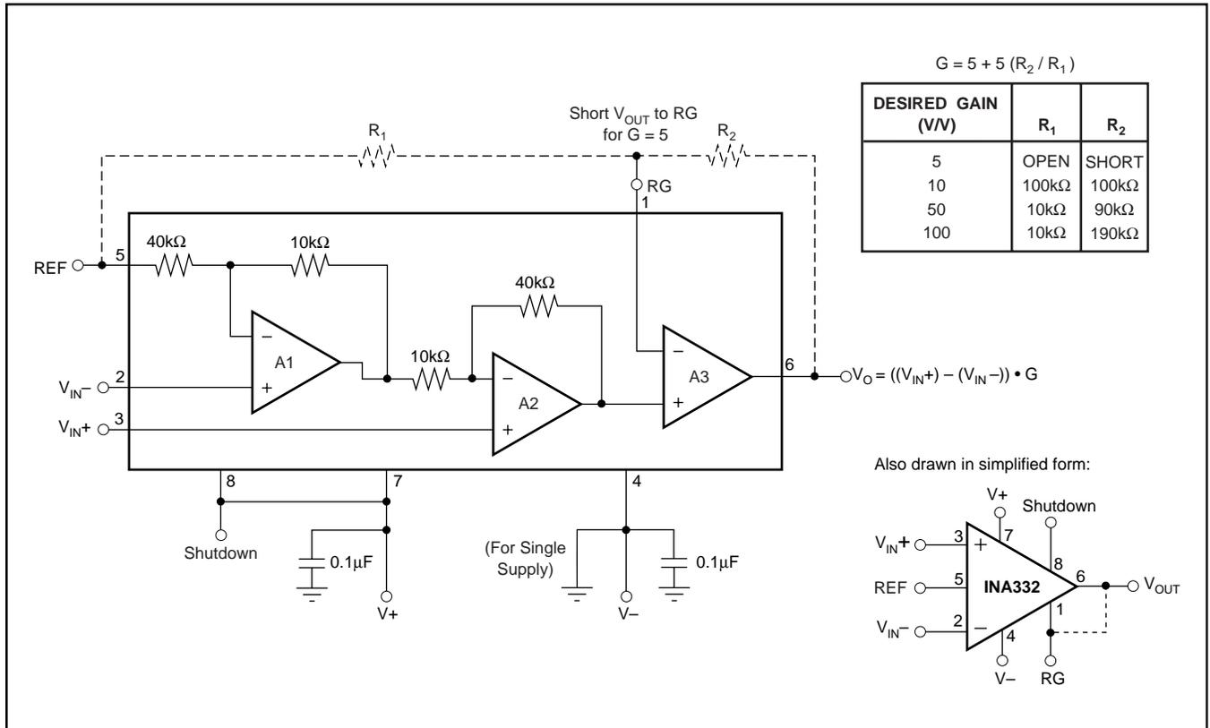
FIGURE 1. Basic Connections.
