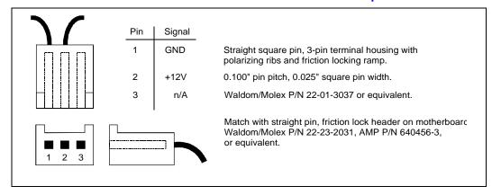
**Table 41. Fan Heatsink Power and Signal Specifications**
