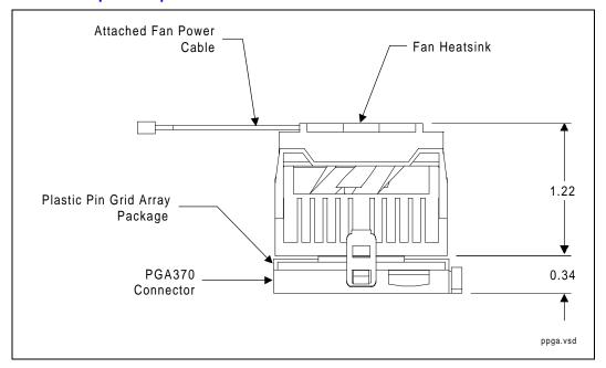
Figure 26. Top View Space Requirements for the Boxed Processor
