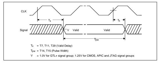
Figure 5. Intel<sup>®</sup> Celeron™ Processor System Bus Setup and Hold Timings
