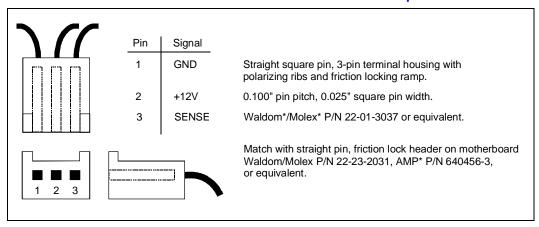
**Table 39. Fan Heatsink Power and Signal Specifications**
