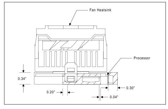
Figure 31. Side View of Motherboard Keepout Requirements
