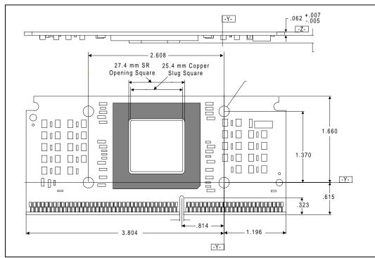
Figure 14. Intel<sup>®</sup> Celeron™ Processor Substrate Dimensions (S.E.P. Package)
