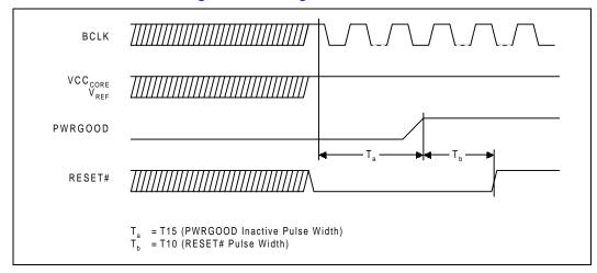
Figure 8. Test Timings (TAP Connection)
