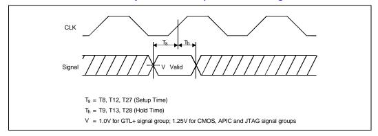
Figure 6. Intel<sup>®</sup> Celeron™ Processor System Bus Reset and Configuration Timings
