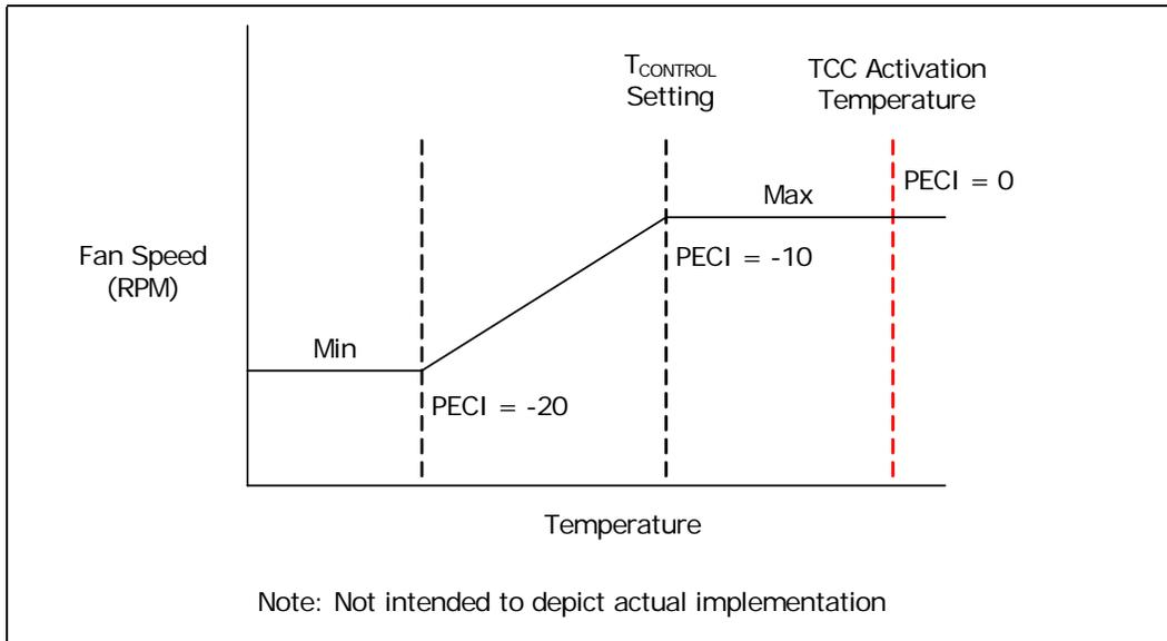
Figure 21. Conceptual Fan Control on Thermal Diode-Based Platforms
