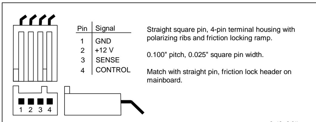
Table 34. Fan Heatsink Power and Signal Specifications
