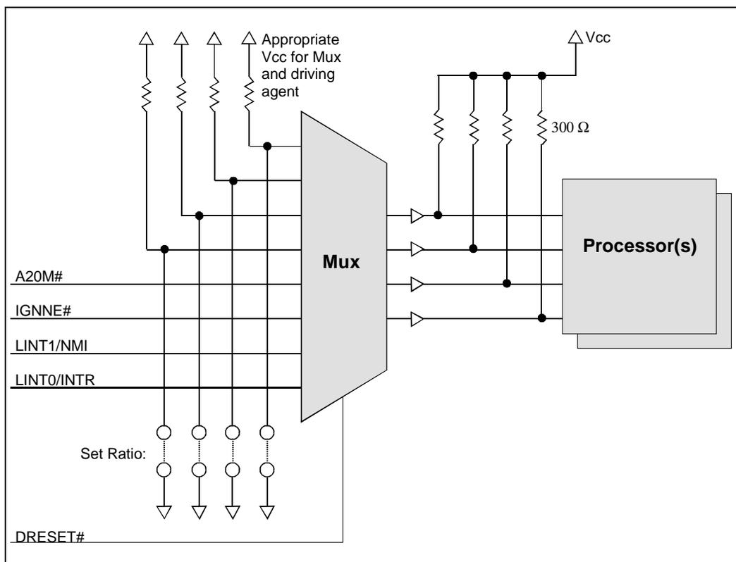
**Note:** Check your chipset documentation to determine if it includes this multiplexing logic for clock ratio pin sharing.
