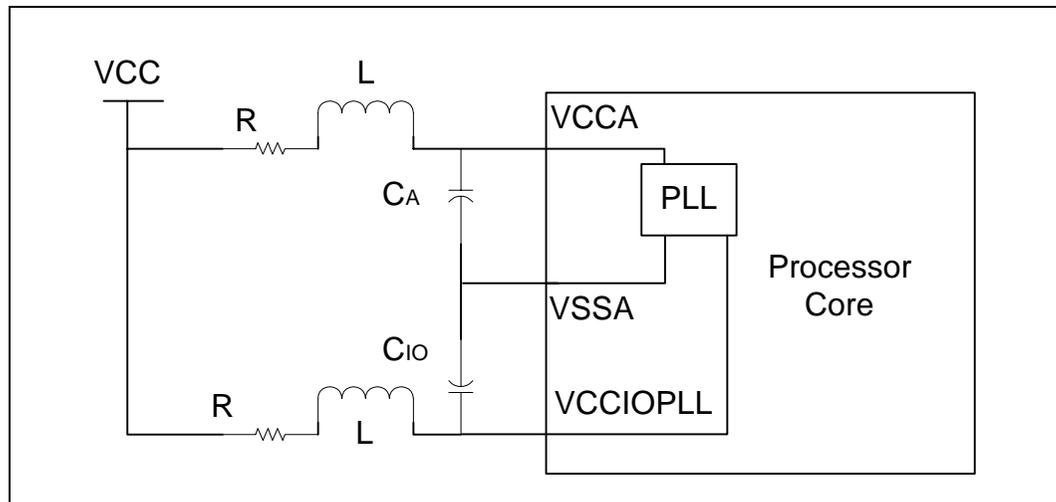
Figure 2. Phase Lock Loop (PLL) Filter Requirements
