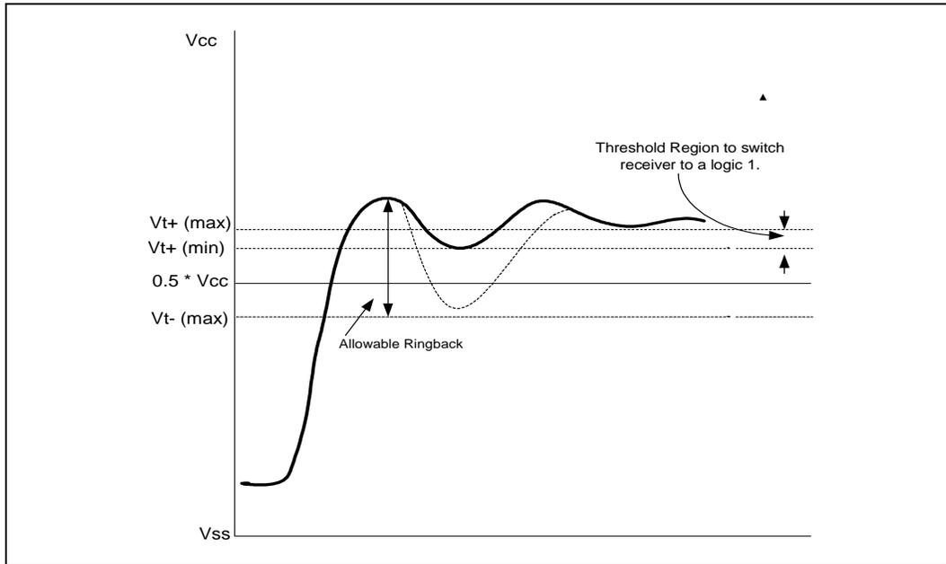
Figure 20. High-to-Low Receiver Ringback Tolerance for TAP Buffers
