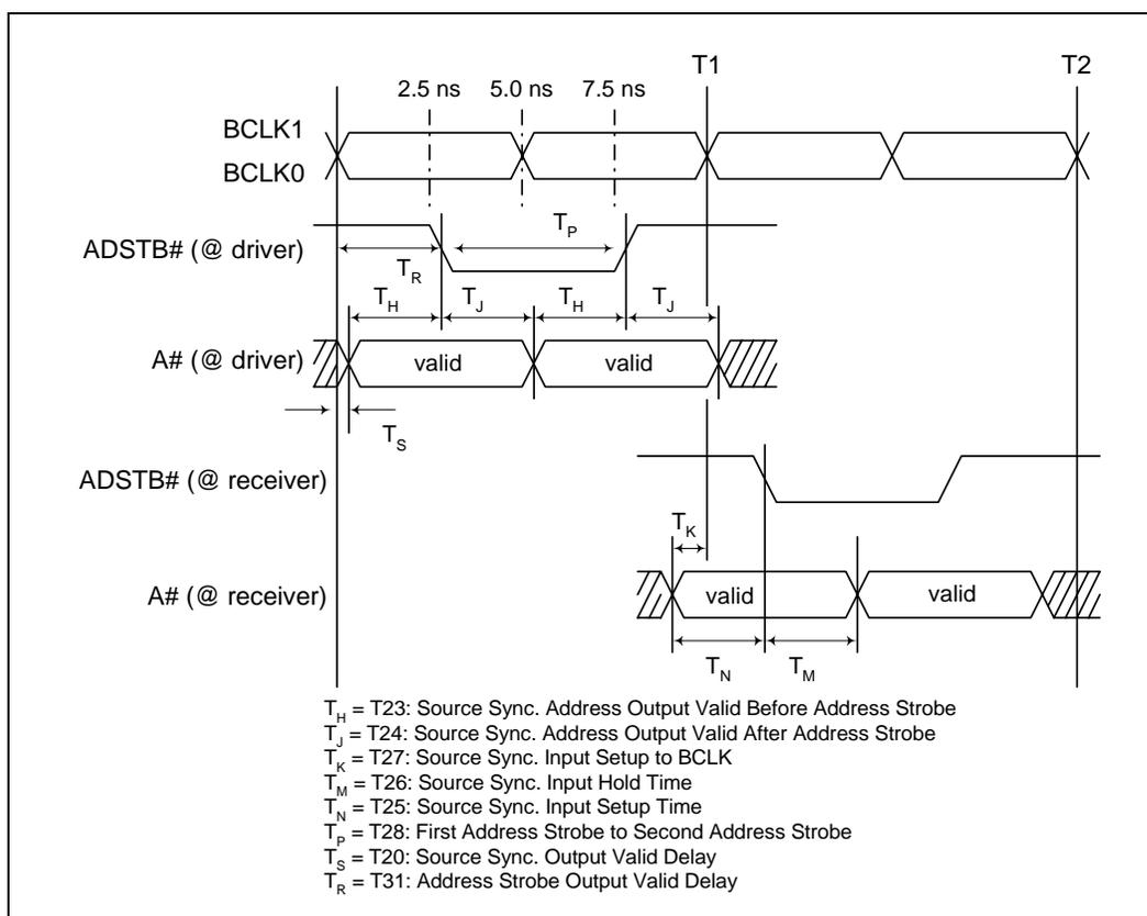
Figure 8. System Bus Source Synchronous 4X (Data) Timing Waveform
