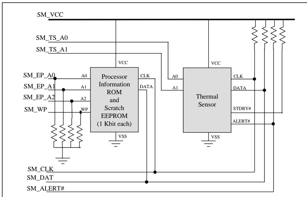
**NOTE:** Actual implementation may vary. For use in general understanding of the architecture. All SMBus pull-up and pull-down resistors are 10 K $\Omega$  and located on the processor.
