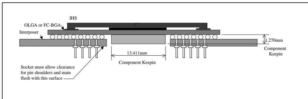
Figure 27. Processor Pin Detail
