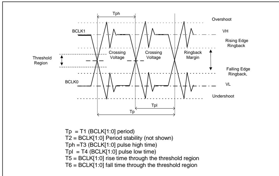
Figure 6. System Bus Common Clock Valid Delay Timing Waveform
