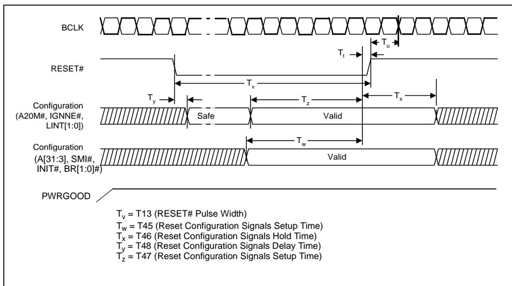
Figure 10. Power-On Reset and Configuration Timing Waveform
