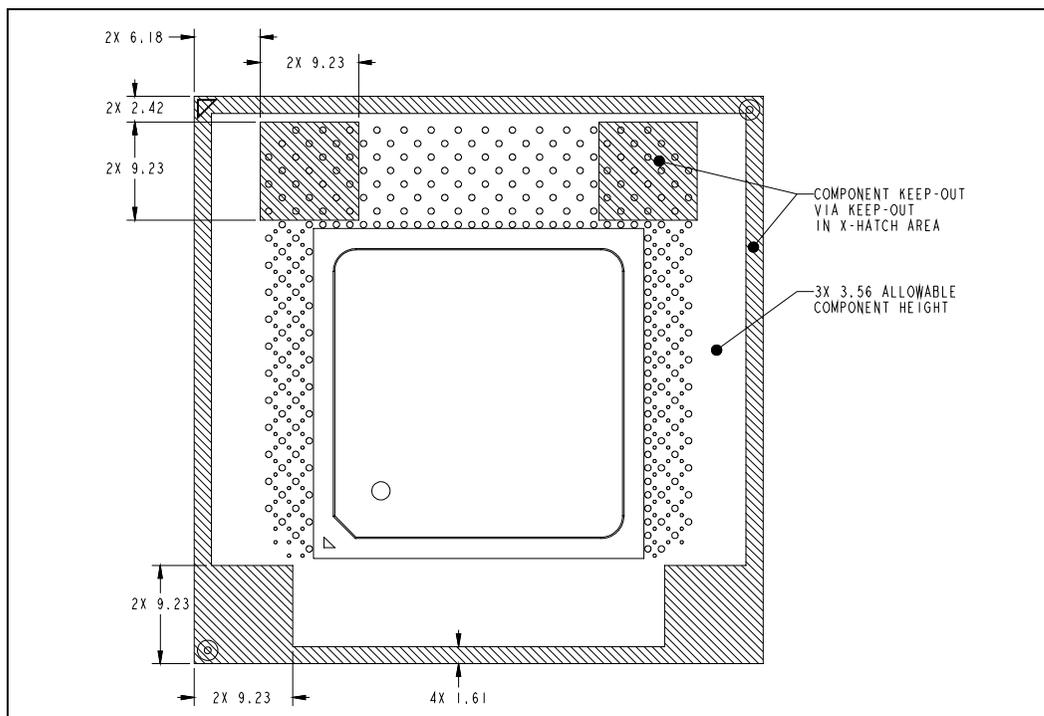
Figure 26 details the keep in specification for pin-side components. The processor may contain pin side capacitors mounted to the processor package. The capacitors will be exposed within the opening of the interposer cavity. This keep-in specification applies to both packages.
