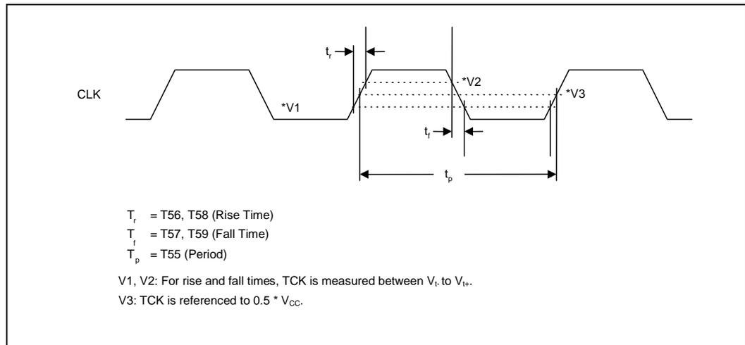
Figure 5. Differential Clock Waveform
