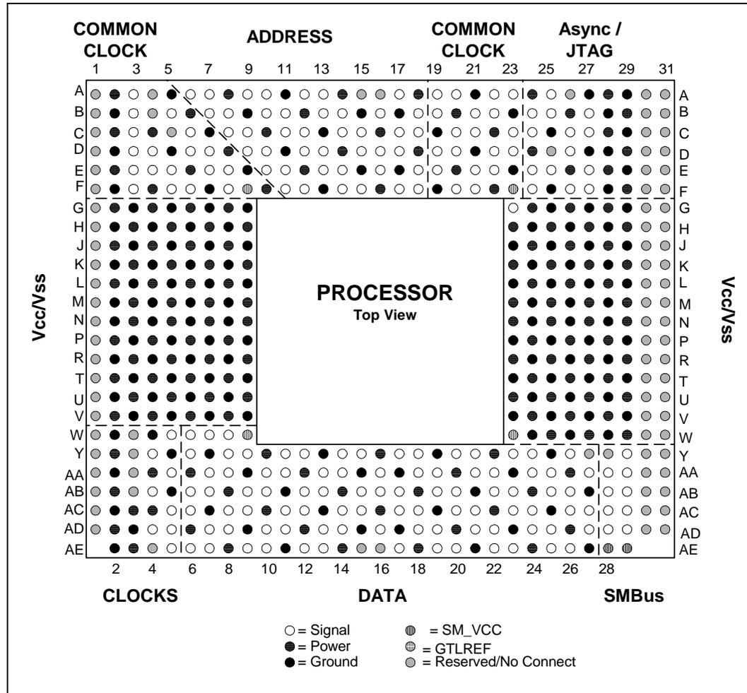
Figure 32. Processor Pin-out Diagram -- Bottom View
