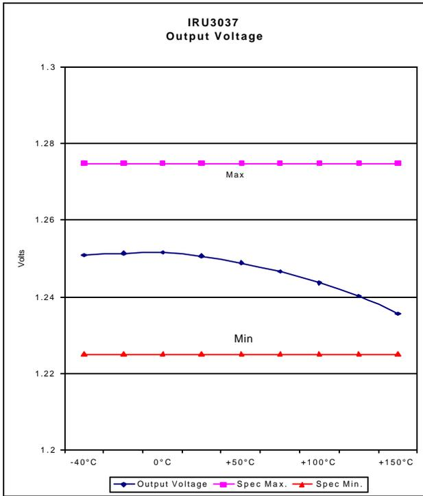
Figure 11 - Output Voltage
