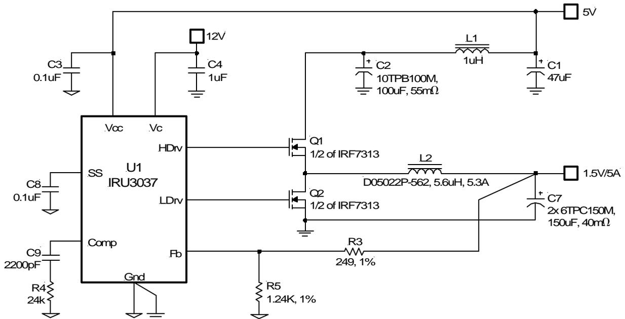
Figure 1 - Typical application of IRU3037 or IRU3037A.
