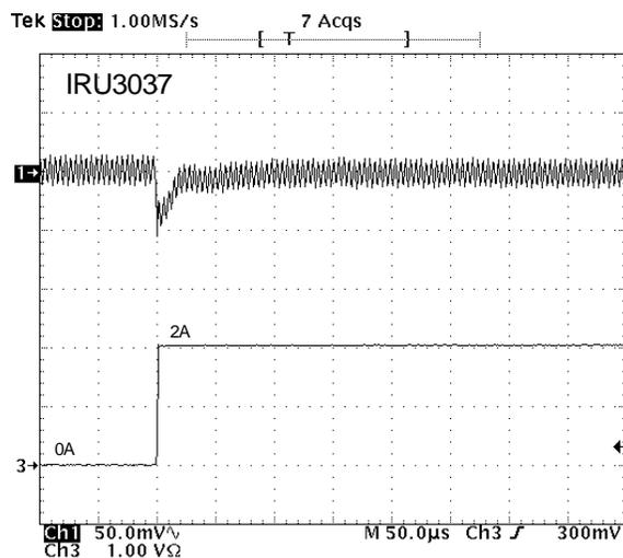
Figure 26 - Transient response @  $I_{OUT} = 0$  to 2A.
