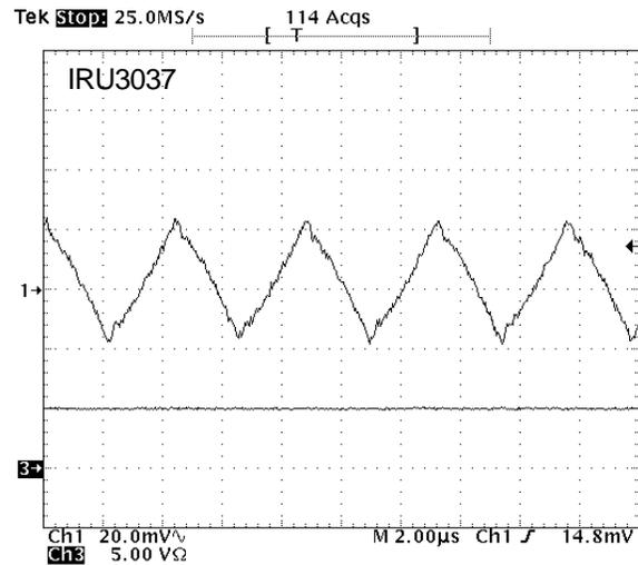
Figure 25 - 3.3V output voltage ripple @  $I_{OUT}=5A$ .
