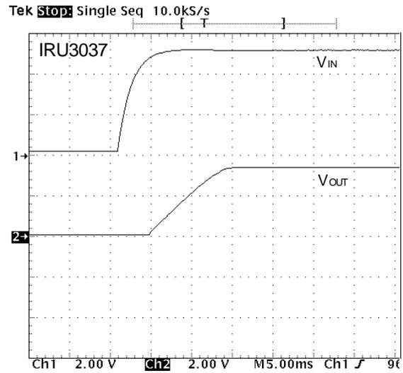
Figure 23 - Start-up time @  $I_{OUT}=5A$ .
