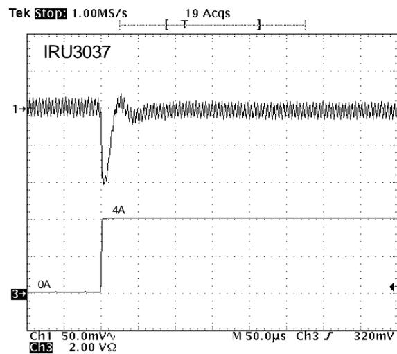
Figure 27 - Transient response @  $I_{OUT} = 0$  to 4A.
