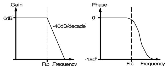
Figure 5 - Gain and phase of LC filter.
