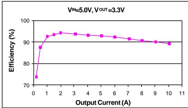
Figure 22 - Efficiency for IRU3037 Evaluation Board.
